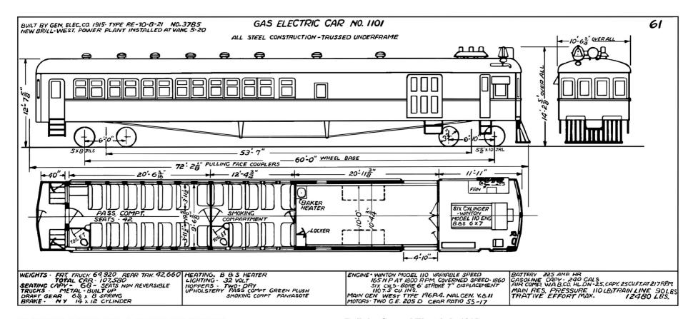
SPOKANE, PORTLAND & SEATTLE RAILWAY 1101 GAS ELECTRIC CAR, 1944 DIAGRAM Scanned and inverted from 1944 Equipment Diagram Book. Restored by Paul T. Hobbs, March 29, 2007 Built by General Electric in 1915 Type RE-70-8-21 Delivered February 19, 1915 New Power Plant installed May 1920 To X-475 April 19, 1944
