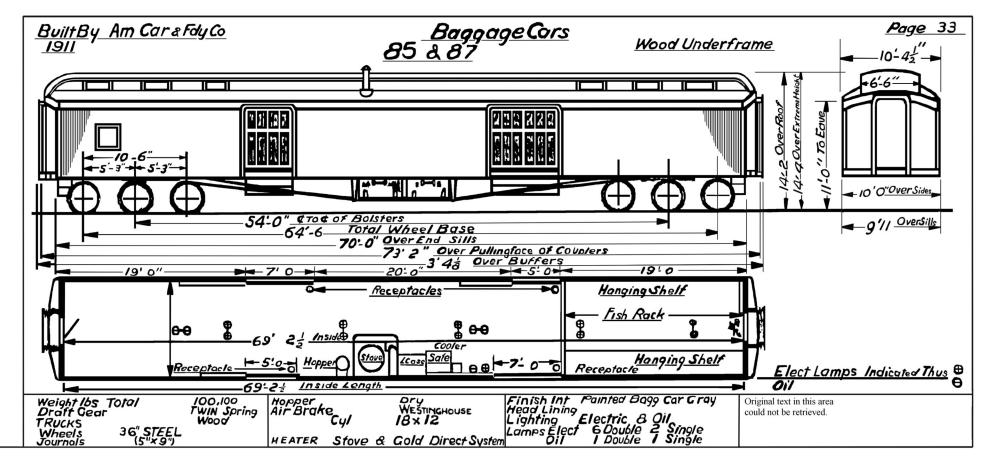
SPOKANE, PORTLAND & SEATTLE RAILWAY 85-87 BAGGAGE CARS, 1926 DIAGRAM Scanned and inverted from copy from Ralph L. Barger. Diagram was extracted from very gray photocopy. Restored by Paul T. Hobbs, May 19, 2006 Built by American Car & Foundry, July 1911 Delivered as Dynamo-Baggage cars. 85 Dynamo to 93 September 1929 85 to X-440 October 11, 1940 86 Destroyed by fire September 9, 1916 86 Dynamo to 70 September 1917 87 Dynamo to 94 July 1930 87 to X-441 October 11, 1940
