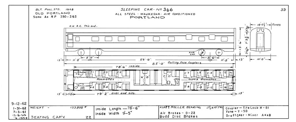
SPOKANE, PORTLAND & SEATTLE RAILWAY 366 SLEEPING CAR, 1962 DIAGRAM Scanned from Passenger Car Diagrams S. P. & S. Ry, PNR/NMRA 1980. Restored by Paul T. Hobbs, October 7, 2006 Built by Pullman-Standard, Plan 4119 Lot 6781, September 1948 Identical to NP 350-363, CB&Q 480-482
