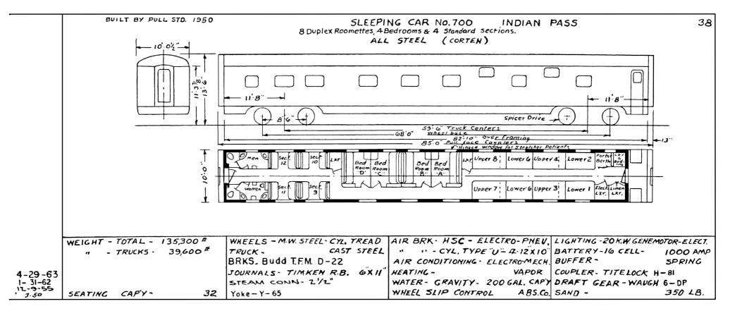
SPOKANE, PORTLAND & SEATTLE RAILWAY 700 SLEEPING CAR, 1963 DIAGRAM Scanned from Passenger Car Diagrams S. P. & S. Ry, PNR/NMRA 1980. Restored by Paul T. Hobbs, May 6, 2006 Built by Pullman-Standard, Plan 4107 Lot 6828 February 1950 Identical to GN 1160 - 1169, 1180 Delivered February, 1950 To BN 1169 (unlikely that number was applied to car) To BN 968242 September 1978
