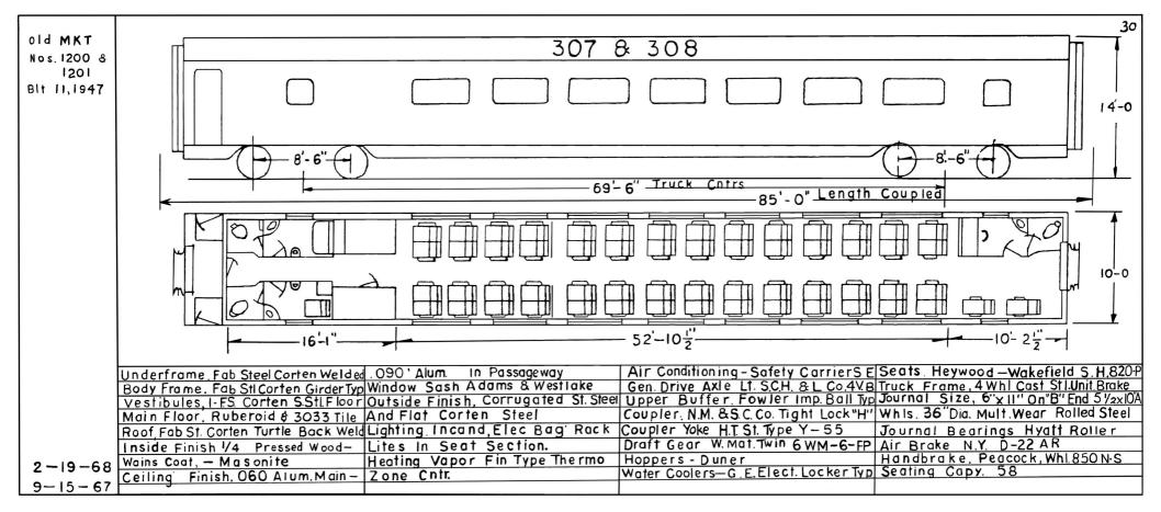
SPOKANE, PORTLAND & SEATTLE RAILWAY 307 - 308 COACH, 1968 DIAGRAM Scanned from Passenger Car Diagrams S. P. & S. Ry, PNR/NMRA 1980. Restored by Paul T. Hobbs, March 14, 2007 Built by Pullman-Standard Plan 7537 Lot 6768, November 1947 As 56-seat Coach with partition, M-K-T 1200, 1201. Operated in "Texas Special", jointly with Frisco (SLSF).
