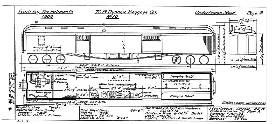
SPOKANE, PORTLAND & SEATTLE RAILWAY 70 DYNAMO BAGGAGE CAR, 1917 DIAGRAM Scanned and inverted from copy from the PNWC Collection. Restored by Paul T. Hobbs, December 14, 1999 Dynamo installed from fire-damaged 86 in September 1917 Dynamo transferred to 92 in July 1929.
