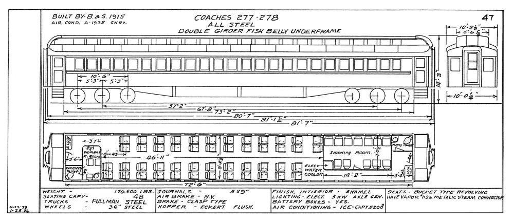
SPOKANE, PORTLAND & SEATTLE RAILWAY 277 - 278 COACHES, 1939 DIAGRAM Scanned and inverted from 1944 Equipment Diagram Book. Restored by Paul T. Hobbs, March 19, 2007 Built by Barney & Smith June 1915 (see diagram 270 - 276 for the as-delivered appearance) Rebuilt and air-conditioned by GN June 1935 Retired December 31, 1968 Served thereafter as cabooses on Portland Astoria line.
