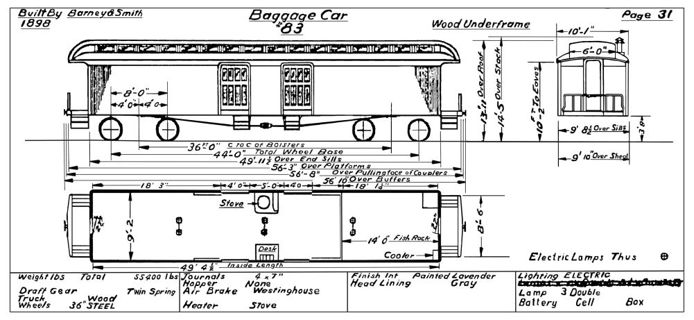
SPOKANE, PORTLAND & SEATTLE RAILWAY 83 BAGGAGE CAR, 1926 DIAGRAM Scanned and inverted from copy from Ralph L. Barger. Restored by Paul T. Hobbs, August 31, 2004 (Here is an example of a diagram in error.)
