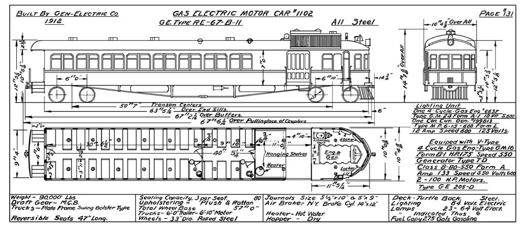
SPOKANE, PORTLAND & SEATTLE RAILWAY 1102 GAS ELECTRIC MOTOR CAR, 1923 DIAGRAM Scanned and inverted from copy from Minnesota Historical Society. Restored by Paul T. Hobbs, January 31, 2005 Built by General Electric and Wason in 1912 as Dan Patch 8 To SP&S 1102 August 31, 1917 To Warren & Ouachita Valley RR #1 Interchanged to Southern Pacific for delivery September 10, 1924.
